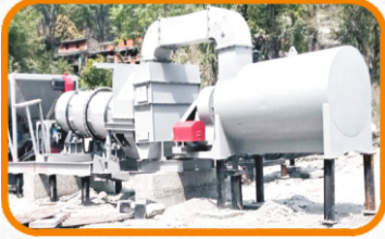
Drum Mix Plant
