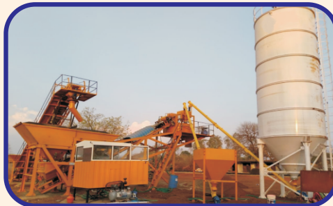
Mobile Concrete Batching Plant
